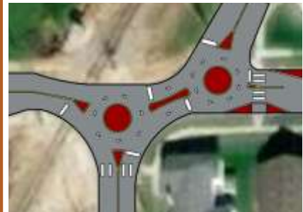
Two mini-roundabouts could improve the 12th/Bardsley/Olive intersection with paint and signage only
