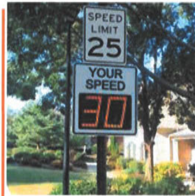
Radar Speed Signs are effective at reducing vehicle speeds. Edge line painting, curb extensions (below), on-street parking and street trees can also reduce speeds.
