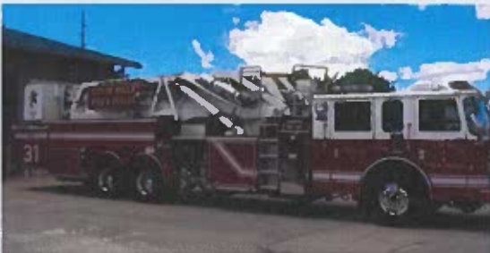
2006 - Dash 95' Platform Pierce $675,000 Purchased used 2011 2,000 gpm pump
